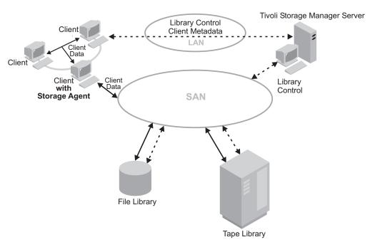
Figure 2. SAN Data Movement with the LANFREECOMMMETHOD option. Solid lines indicate data movement. Broken lines indicate movement of control information and metadata. The LANFREECOMMMETHOD option allows the storage agent to support several clients while installed on only one of the clients.
